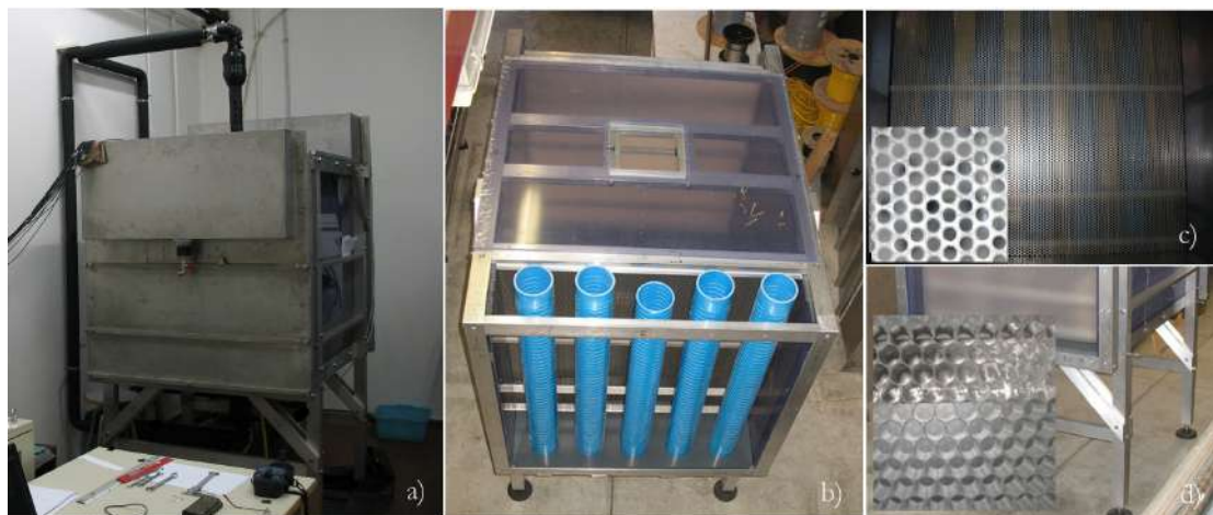
Figure 2 a) The experimental apparatus in test configuration. The insulated circuit of the copper heat exchanger is visible; b) A view from the top of the filtration fluid inlet tank with the micro-pitted pipes; c) The perforated stainless steel wall; d) A detail of the flow rectifier located between the micro-pitted pipes and the perforated wall.
